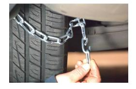
6. Drive forward one car length, then check the chain and hand tighten again if needed and/or possible. Repeat this step to ensure chains remain tight.
