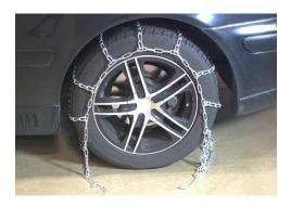
5. Hand tighten the fastener and secure to the side rail. Cut or wire up any excess tail Links if needed.
