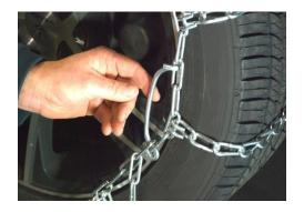
3. Reach to back of tire and fasten the inside hook end to the tail link.
