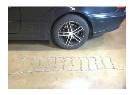
Thread the fastener thru the tail link after pulling chain tight. If extra tail links, thread onto fastener as well.
