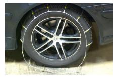
6. Hand tighten the cable and fasten.
